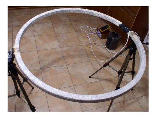
This set is suitable for immunity testing towards durable and transient magnetic field of mains frequency 50 (60) Hz. The magnetic field is manually settable on variable voltage transformer, while the current in coil is checking by ammeter in accordance with the conversion table. The coil has many turns and is holding by two camera stands making possible rotation along horizontal axis.
